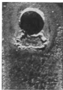
FIG. 6. Pitting of Aluminum Brass around supports in recirculated water to which silt was added at Harbor Island.
