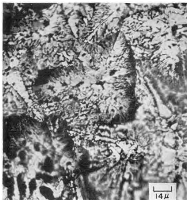
FIG. 2. Appearance at vertical surface of chill cast lead-antimony ingot after etch with acetic acid-hydrogen peroxide solution. Antimony (light areas) covers almost the entire surface and shows primary crystallization although representing only 5% of the total alloy. 500X.
