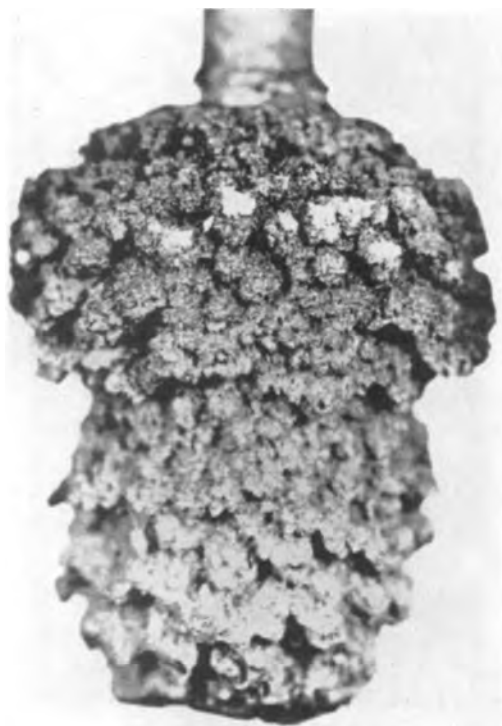
Fig. 7 Typical electrolytic zirconium deposit. (Reduced one-third in reproduction)
