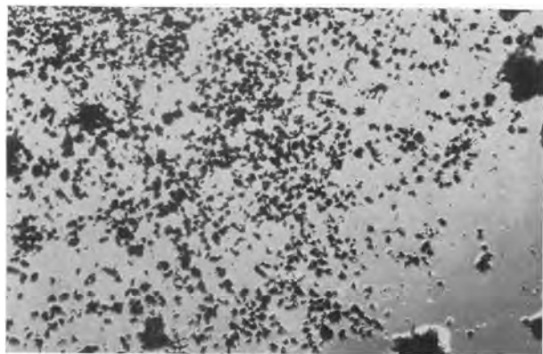
FIG. 10. Molybdenum powder from 100-gram batch produced at 600°C from bath B. 50X.
