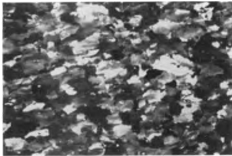
FIG 24 Electrolytic zirconium metal, arc-melted and hot-rolled 80% from 0.375-0.07 in., at 700°C followed by 40% cold reduction from 0.070-0.030 in. Polarized light. 250X
