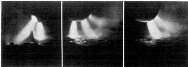
FIG. 2. Arc in a melting furnace. Three consecutive frames of a movie taken at a speed of 16 frames/sec.
