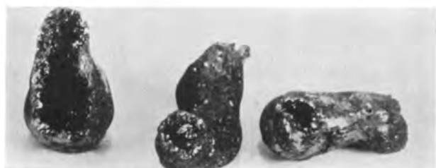
FIG. 3. Vermiculate Be 2 C. Top—core of high-temperature heat; bottom—individual tubes showing hollowness.
