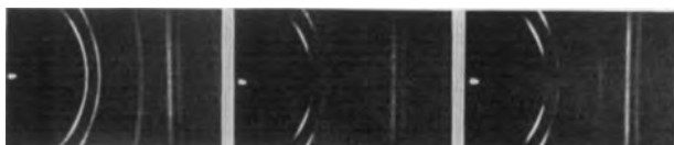
FIG. 8. X-ray diffraction patterns of copper deposits. Electrolyte: 0.17M \text{CuSO}_4 + 0.02M \text{H}_2\text{SO}_4 ; current density: 20 ma/cm 2 ; plating time: approx. 70 min. Pattern a (left), with quiescent solution; pattern b (center), with stirring; pattern c (right), with progressive ultrasonic waves (1000 kc/sec, 4 watts/cm 2 ).
