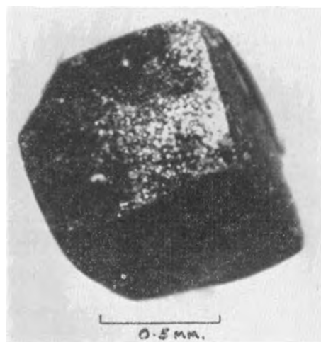
FIG. 3. Shape of the solid obtained by partial dissolution of a germanium globule.
