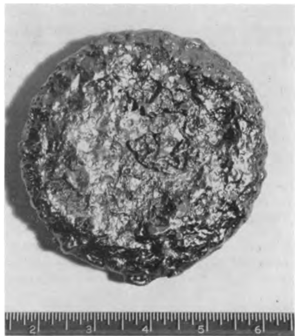
FIG. 1. Vanadium button produced by bomb reduction of V_2O_5 with calcium.
