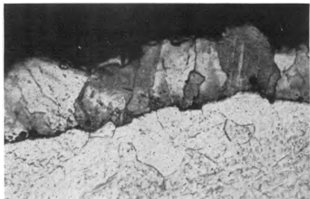
FIG. 4. Cross section of adherent molybdenum layer after removal of overlying powder—bath A. 500X.
