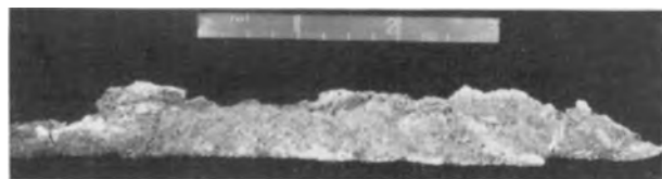
FIG. 2. Photograph of an ingot of calcium carbide produced in the horizontal continuous-ingot furnace. (Ingot was moved from right to left under the electrodes.)
