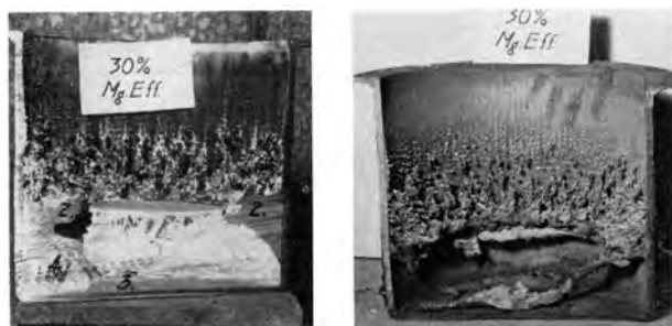
FIG. 2. Bisected chamber after 30% reduction. Left, undistilled segment; right, distilled segment.
