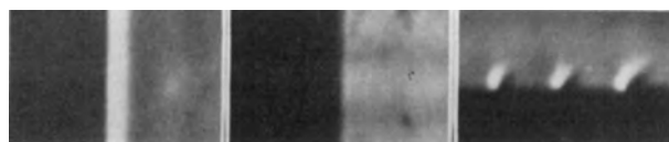
FIG. 9. Schlieren photographs of concentration gradients at copper cathode. Electrolyte: 0.86M \text{CuSO}_4 + 0.02M \text{H}_2\text{SO}_4 ; current density: 25 ma/cm 2 . Fig. 9a (left): vertical cathode without ultrasonic waves. Fig. 9b (center): vertical cathode with progressive ultrasonic waves (1 watt/cm 2 at 1000 kc/sec). Fig. 9c (right): horizontal cathode with standing waves ( \approx 0.1 watt/cm 2 at 1000 kc/sec).
