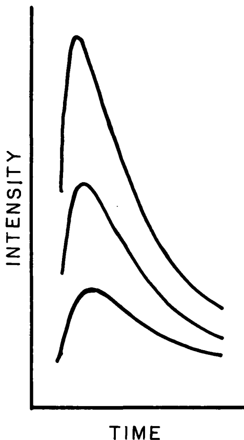
FIG. 1. Triply exposed oscillogram for blue electroluminescence, square wave fields, 90 cps, 250 \mu sec rise time.
