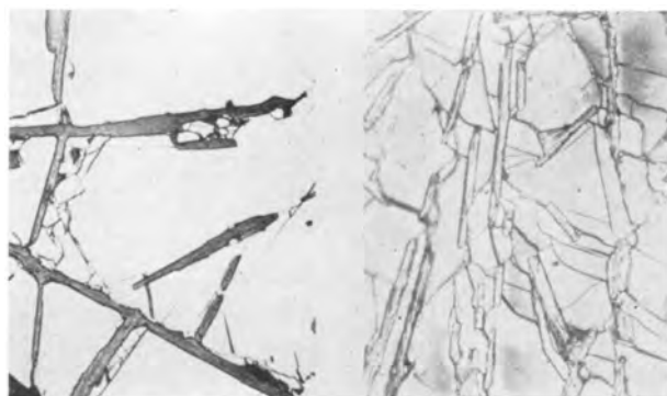
FIG. 4. Graphite flakes in a \text{Be}_2\text{C} matrix. Left, unetched, right, air etched.
